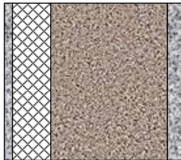
Pavimento:  $U_{pav.} = 0.5 \text{ W/m}^2 \text{ k}$
